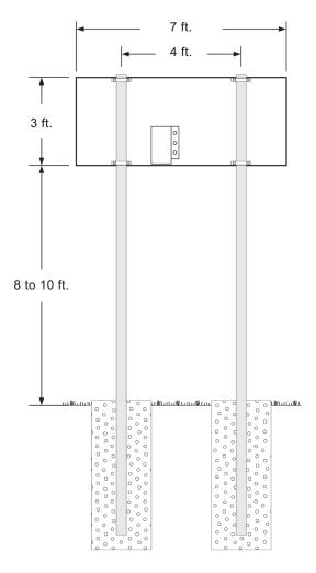
Once you have verified the position of the posts and the size of the footings, you are ready to dig your holes, pour your concrete, and set your posts. There are several techniques for ensuring proper alignment of the posts. Typically installers will construct a temporary wooden support frame to hold the posts in place while the concrete sets. Having plumb posts in the proper position is the key to a smooth mechanical installation.
